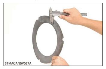
1. Measure the brake plate thickness with vernier calipers.
