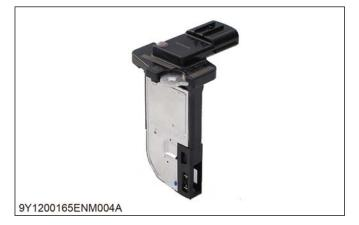
The amount of air intake required for control of the EGR valve used to reduce NOx is measured.
