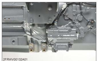
(6) Shuttle valve delivery pipe
