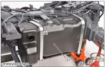
(1) Fuel lever sensor connector (2) Fuel tank
