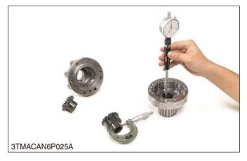
1. Measure the differential side gear boss O.D.
