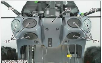
(19) Steering shaft cover (20) Panel under cover (R.H.) (21) Air outlet
