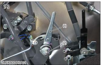
(1) Hand accelerator lever(2) Locking nut
