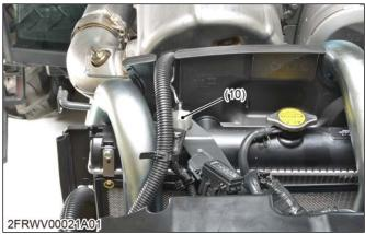
(10) SCR temperature sensor connector
