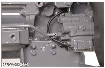
(1) Hydraulic shuttle delivery pipe
