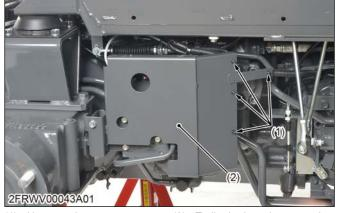
(1) Harness clamp (2) Trailer brake valve protection cover
