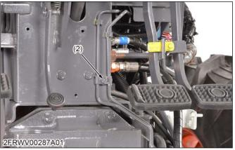
(2) Brake pipe clamp mounting bolt
