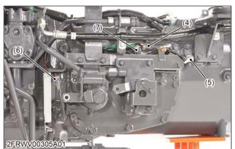
Main gear shift (6th) switch (4)connector Shuttle rotation sensor con-
