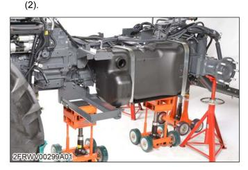
5. Remove the front and rear support mounting bolts and nuts (4), (5) of fuel tank (2).
