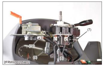
(7) Combination lever switch connector(8) Combination lever switch
