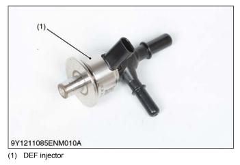
DEF (Diesel Exhaust Fluid) is injected into a mixing pipe.
