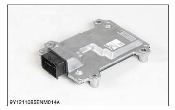
The ACU communicates with the ECU via CAN communication.
