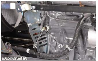
(1) Engine oil pressure switch (2) Connector (Harness side)
