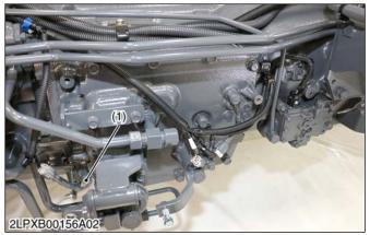
(1) Gear lock parking detect switch
