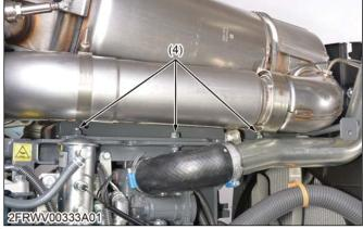
(4) SCR muffler bracket mounting bolt and nut
