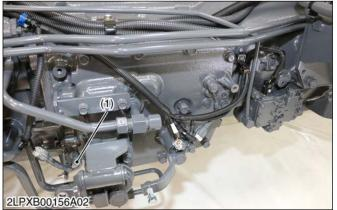
(1) Gear lock parking detect switch
