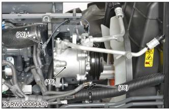
(18) Ground wire mounting screw (20) Compressor 1P connector (19) Compressor
