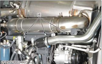
(4) SCR muffler bracket mount-
