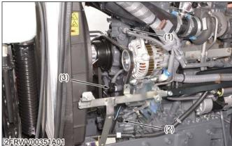
Coolant temperature sensor (1)connector Crankshaft position sensor (2)
