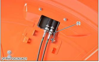
Auxiliary control lever brack-(5) et
