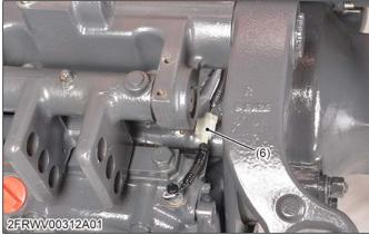
(6) PTO speed detect switch connector
