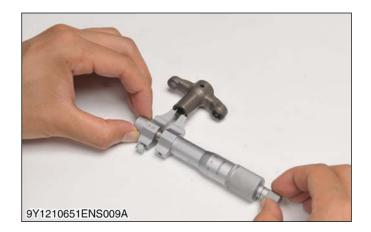
1. Measure the valve bridge arm I.D. with an internal micrometer.
