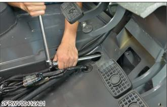
(1) Engine and clutch housing (2) Grommet mounting nut
