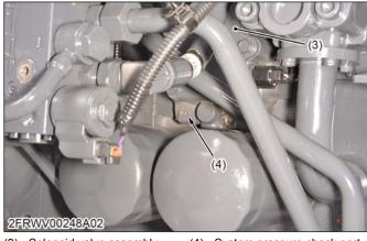
(3) Solenoid valve assembly (4) System pressure check port plug
