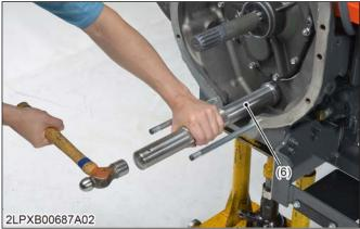
(6) Propeller shaft oil seal fitting tool
