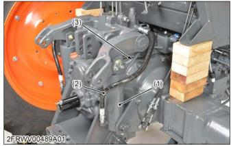
(1) Hydraulic cylinder(2) Hydraulic cylinder delivery
