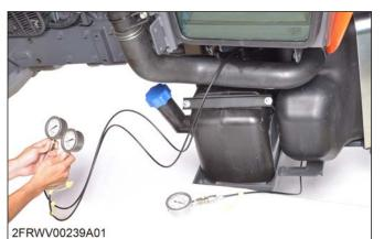
Shuttle lever Clutch pedal F port pressure R port pressure M port pressure Fully pressed 0 0 2.06 to 2.25 MPa Forward Free 21.0 to 22.9 kgf/cm<sup>2</sup> 0 299 to 326 psi 2.06 to 2.25 MPa 21.0 to 22.9  $kgf/cm^2$ Fully pressed 0 0 229 to 326 psi 2.06 to 2.25 MPa Reverse 21.0 to 22.9 kgf/cm<sup>2</sup> 0 Free 299 to 326 psi Less than 0.28 MPa Neutral 0 0 2.9 kgf/cm<sup>2</sup> 41 psi
