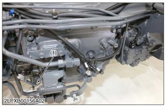
(1) Gear lock parking detect switch
