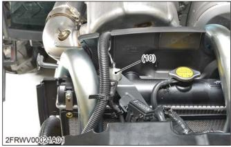
(10) SCR temperature sensor connector
