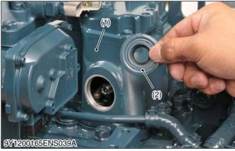
(2) Injector oil seal (1) Cylinder head cover 1
