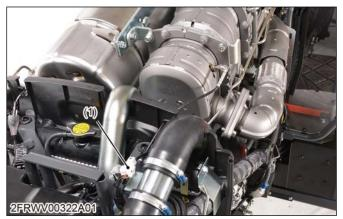
(1) Exhaust temperature sensor (T2) connector
