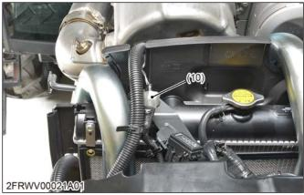
(10) SCR temperature sensor connector
