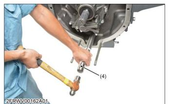
(4) Propeller shaft sleeve fitting tool
