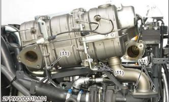
(11) DPF muffler mounting bolt and nut
