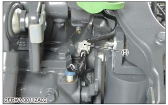
(5) PTO speed detect switch connector
