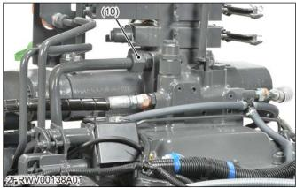
(10) 3-point hitch delivery pipe 2 mounting nut
