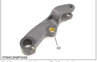
(1) Lift arm support bushing (2) Lift arm bushing
