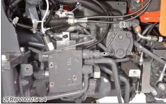
Solenoid valve delivery pipe (8)
