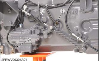
Shuttle valve spool neutral (3) Shuttle solenoid connector (1)switch connector
