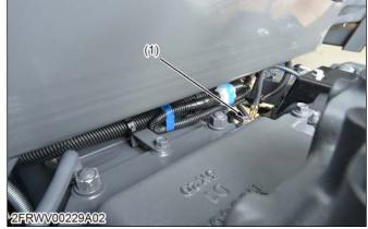
(1) Grounding cable mounting bolt
