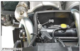
(10) SCR temperature sensor connector
