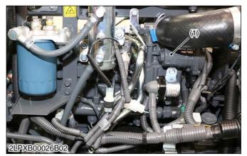
(2) (1) Intake throttle valve (2) Connector (Harness side)
