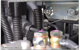
(5) Brake pipe (R.H.) (6) Brake pipe (L.H.)
