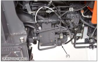
(6) Trailer brake pressure switch (7) Solenoid valve connector
