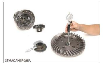
1. Measure the bore I.D. of the differential case and 35T bevel gear.
