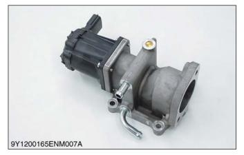
This is a device that regulates EGR gas flow. The degree the valve is open is detected using a lift sensor and a motor is used to set this to the degree of open calculated using signals including the engine speed. Also, passing engine coolant through the housing enables controlling temperature rise of the EGR valve.
