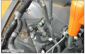
(1) Gear lock parking lever switch
