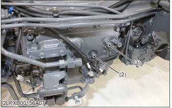
(1) Main gear shift switch (6th) (2) Range gear shift switch (Hi)
