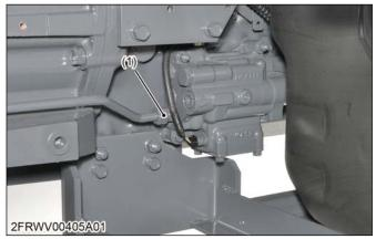
(1) Shuttle valve delivery pipe
