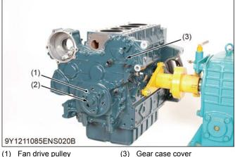
(1) Fan drive pulley (2) Crankshaft screw
