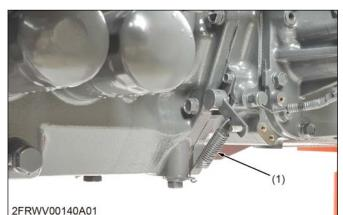
(1) Gear lock parking brake re-
