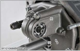
(5) Internal circlip
