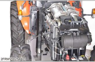
(1) Muffler pipe(2) Muffler pipe fixing bolt
