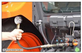
If the pressure is not within the factory specification, adjust the relief valve adjuster (3).
