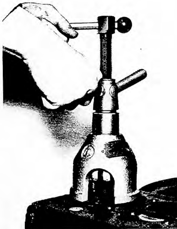
FIG. 116 REMOVING VALVE SEAT INSERT SERVICE TOOL MF540
