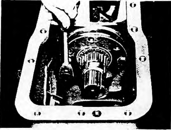
FIG. 12 REMOVING DRIVING PINION ASSEMBLY
