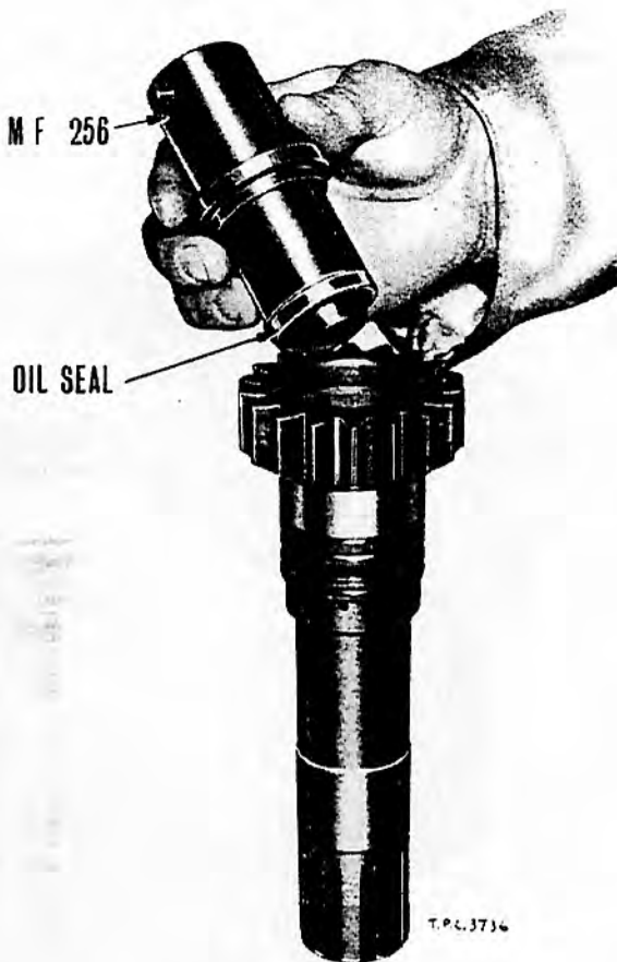
FIGURE 36. FITTING MAIN DRIVE SHAFT PINION OIL SEAL
