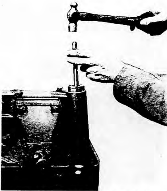
FIGURE 7 EXPANDING THE SPINDLE BUSHES
