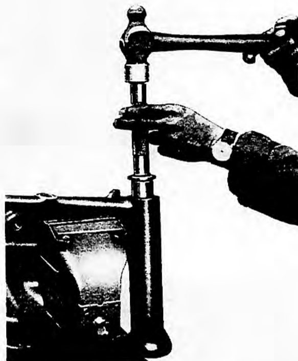
FIGURE 6 FITTING NEW SPINDLE BUSHES
