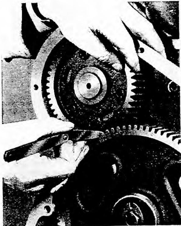
FIGURE 20 CHECKING CAMSHAFT AND IDLER GEAR BACKLASH
