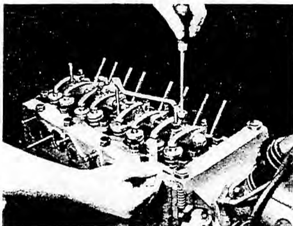
FIG. 121 SETTING VALVE TIP CLEARANCES
