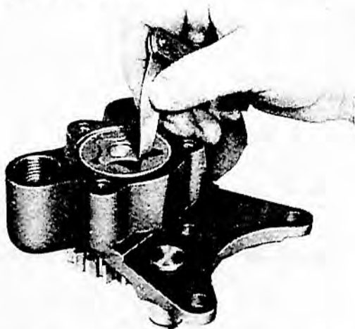
FIGURE 16 CHECKING CLEARANCE BETWEEN DRIVING AND DRIVEN ROTOR
