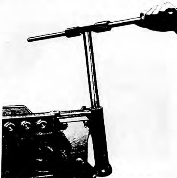
FIGURE 8 REAMING SPINDLE BUSHES
