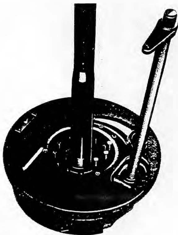
FIGURE 60 REPLACING HALF SHAFT
