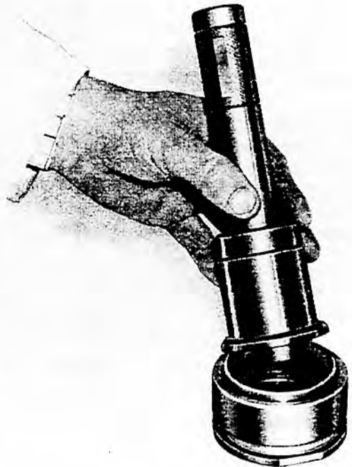
FIGURE 9. REPLACING P.T.O. OIL SEAL IN OIL SEAL RETAINER
