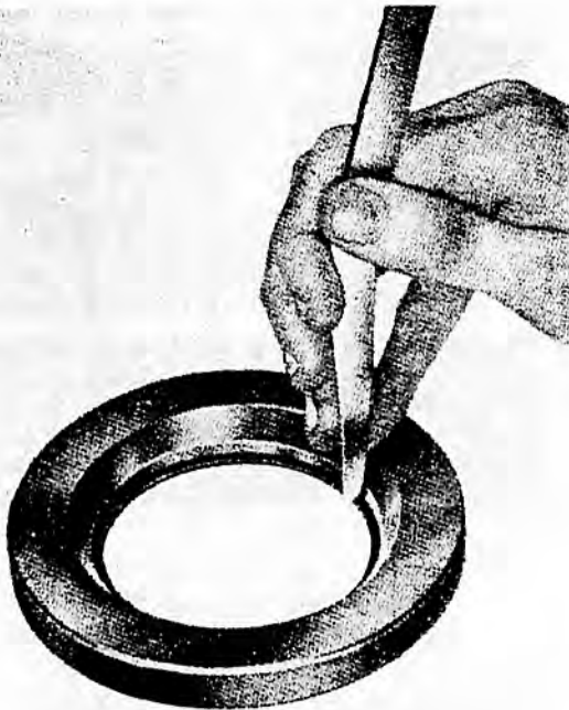
FIG. 136 CHECKING PISTON RING GAP USING RING GAUGE MF185
