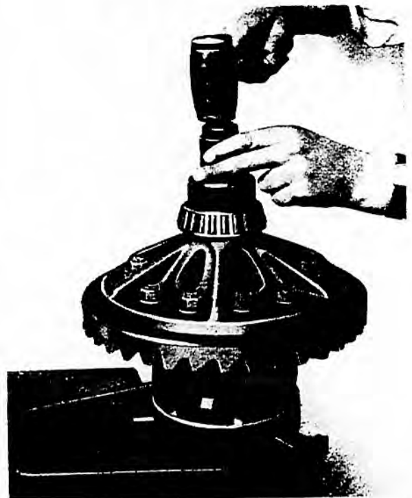
FIG. 28. REPLACING DIFFERENTIAL BEARING CONES
