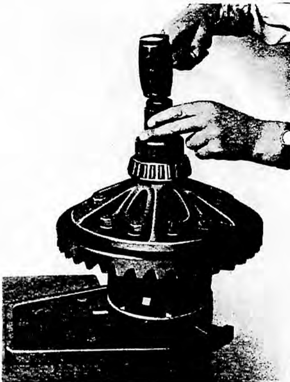
FIG. 15 REPLACING DIFFERENTIAL BEARING CONES
