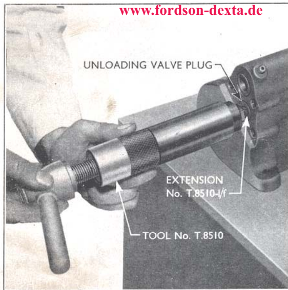
Fig. 21 Removing Unloading Valve Plug
