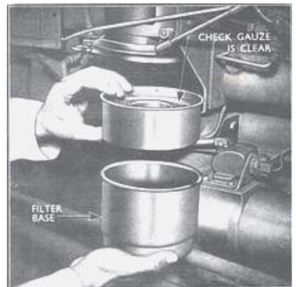
Fig. 4 Removing the Air Cleaner Base
