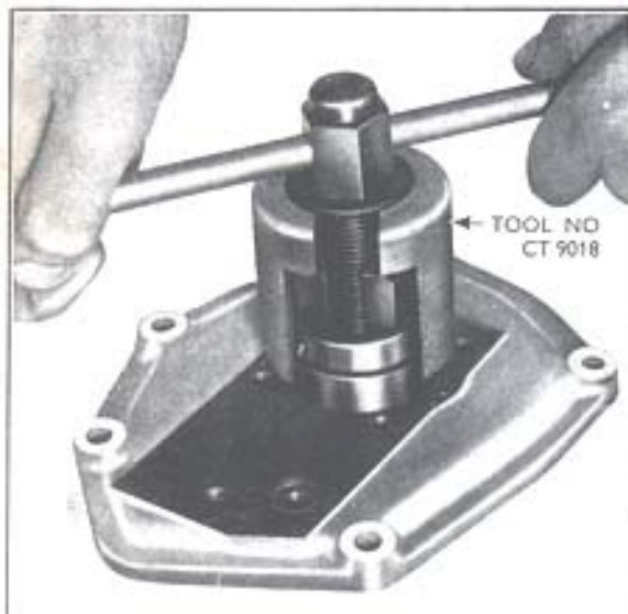
Fig. 14 Removing the Camshaft Outer Races
