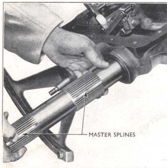
Fig. 36 Assembly of Lift Cross-shaft to Cover
