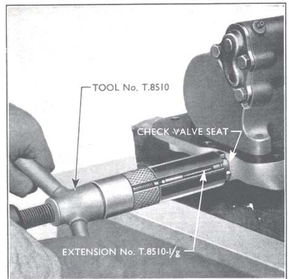
Fig. 17 Removing Check Valve Seat
