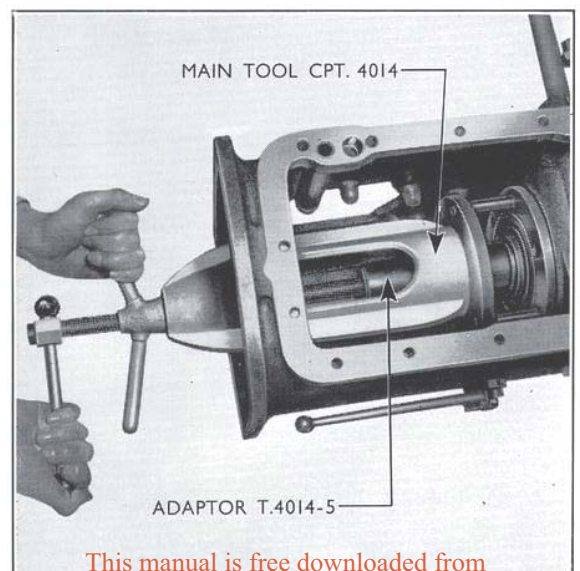
Fig. 23 Withdraw the Drive Pinion Assembly
