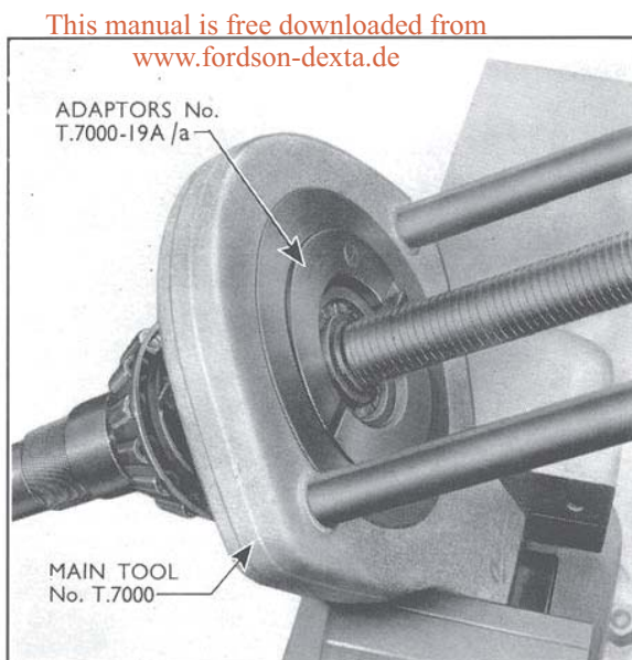
Fig. 24 Removing the Pinion Pilot Bearing
