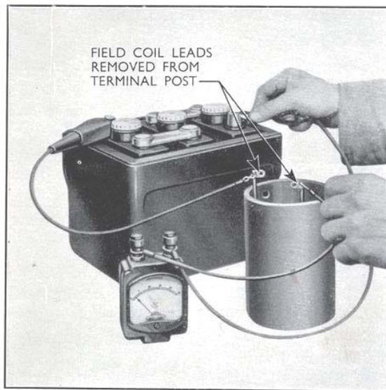
Fig. 5 Testing Field Coils for Continuity
