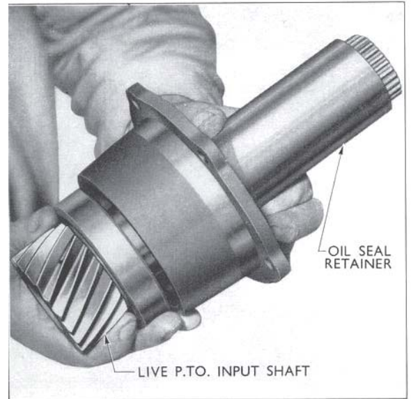
Fig. 3 Refitting P.T.O. Input Shaft
