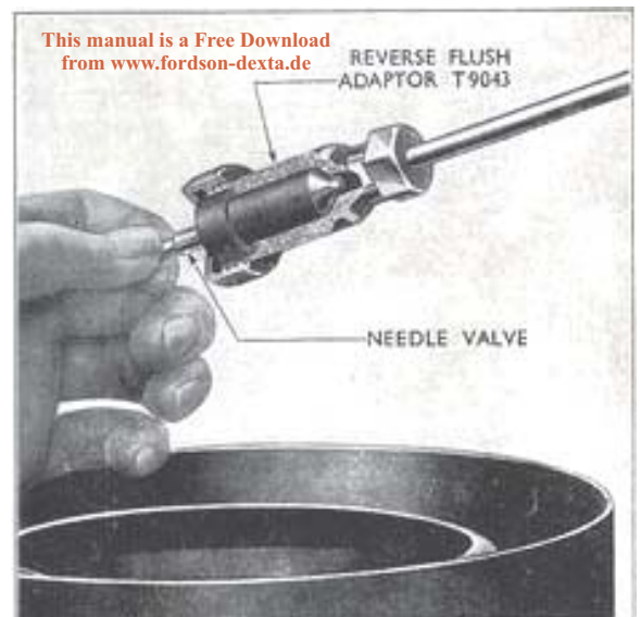
Fig. 29 Reverse Washing the Nozzle
