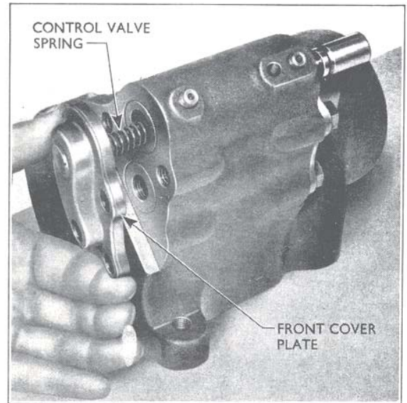
Fig. 27 Replacing Cylinder Front Cover Plate
