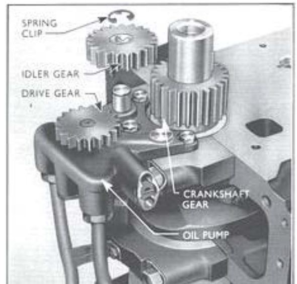
Fig. 31 Oil Pump and Idler Gear
