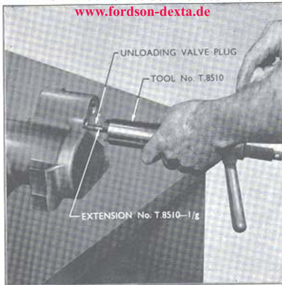
Fig. 53 Removing the Unloading Valve Plug
