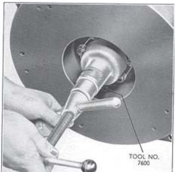
Fig. 19 Removing Clutch Pilot Bearing
