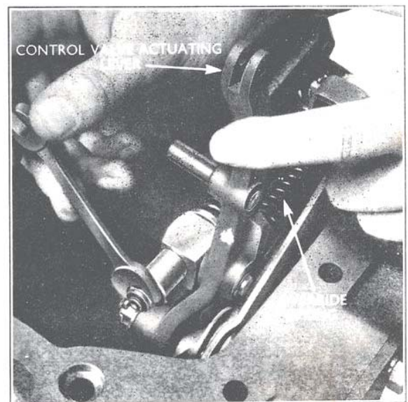
Fig. 35 Retention of Qualitrol Link to Swivel
