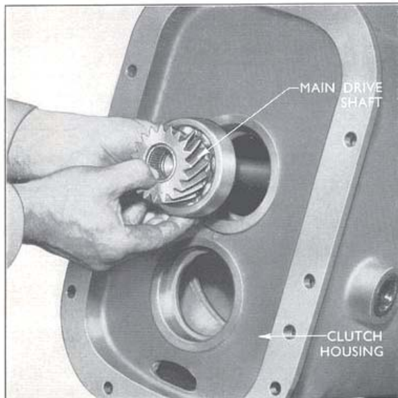
Fig. 7 Removing Main Drive Shaft
