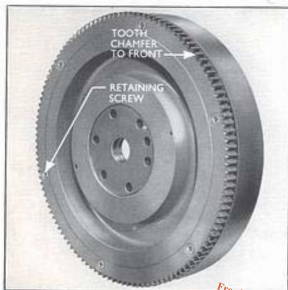
Fig. 17 Flywheel and Ring Gear
