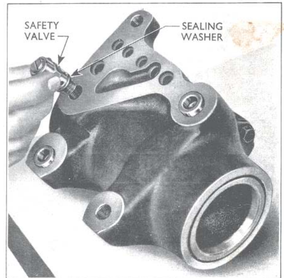
Fig. 28 Replacing Ram Cylinder Safety Valve
