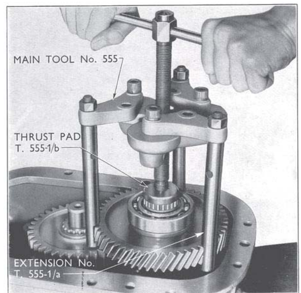
Fig. 17 Removing Main Countershaft Gear and Bearing
