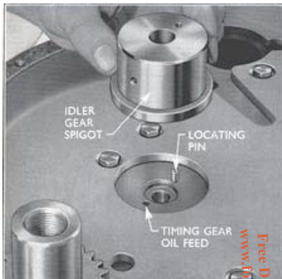
Fig. 10 Idler Gear Spigot
