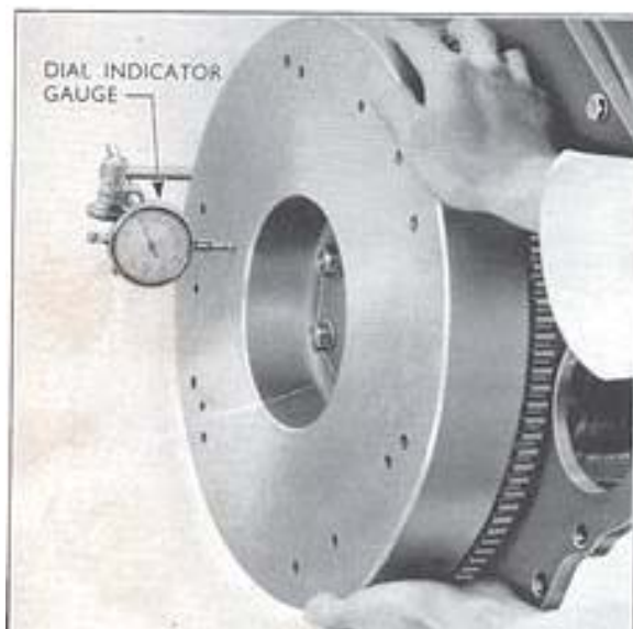
Fig. 18 Checking Flywheel "Run-Out"
