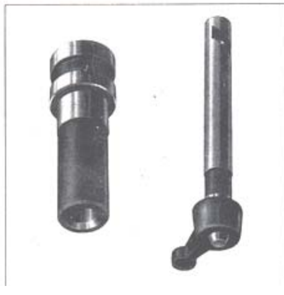
Fig. 10 Injection Pump Element
