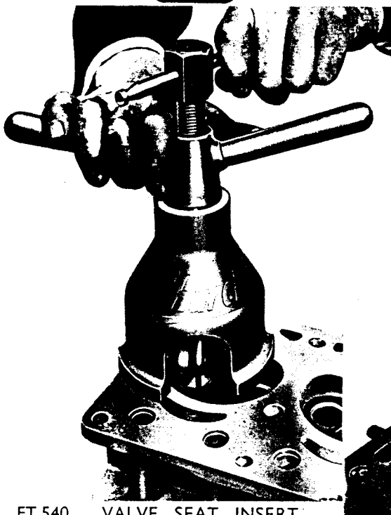
FT.540 VALVE SEAT INSERT REMOVER (TE-20 only) Removes Valve Seat insert Part No. 1678
