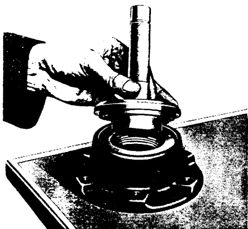
FT.29. REAR HUB OIL SEAL DRIVER for replacement of oil seal Part No. 1082
