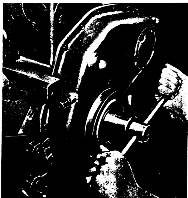
FIG. 126. REMOVING STARTER JAW. SERVICE TOOL FTB. 16.
