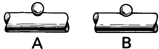
Figure 9. SELECTOR ROD AND DETENT BALL A. Correct B. Incorrect
